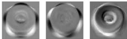
Figure 8: The first three *eigenimages*  $e_1, e_2, e_3$  serve as image feature mask for the rotational part of the PCA-system (see also Sec. 2.2) [7].
