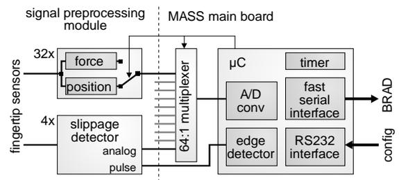
Fig. 10: **Diagram of MASS (*Multi-channel Analog Signal Sampler*):** The microcontroller gathers data from the sensors according to a configurable scan list and sends this data to BRAD via a fast serial line.
