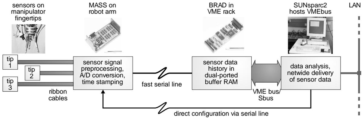
Fig. 9: **Diagram of the experimentation system:** Two components developed at our laboratory, MASS and BRAD, link the fingertip sensors to a standard workstation. MASS handles sensor sampling while BRAD ensures fast data transfer by means of dual-ported memory.
