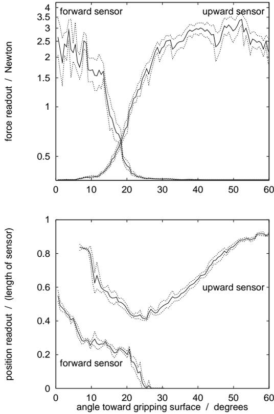
Fig. 6: **Simultaneous force and position traces of two sensors during a rolling movement:** Angles of  $0^\circ$  and  $45^\circ$  correspond to a parallel alignment of the contact surface with the forward and the upward sensor, respectively. When rolling over the polyhedron's edge, the upward sensor smoothly takes over from the forward sensor to produce reliable output throughout the whole movement.
