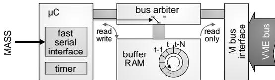
Fig. 11: **Diagram of BRAD (Buffered Random Access Driver):** The microcontroller receives data packets from MASS and maintains a ringlike history buffer. This buffer can be accessed at random from all VME busmaster devices.
