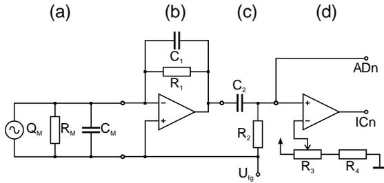
Fig. 3: **Amplifier circuit for one PVF<sub>2</sub> sensor:** The equivalent circuit for the sensor (a) shows the similarity to a capacitive microphone. A charge amplifier (b) and a first-order high-pass filter (c) produce the analog signal. The pulses generated by the threshold comparator (d) are subsequently analyzed by an edge detector.
