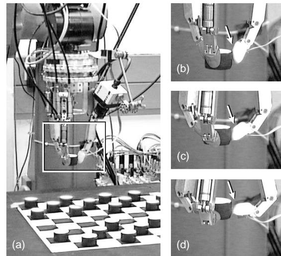
Fig. 1: **Hydraulic hand mounted on robot arm:** A typical sequence is shown where force sensing is needed while rolling over the contact surface (b–d). The fingers have human-like degrees of freedom: a cardanic base joint for sideward and inward bending and two coupled joints for flexing.
