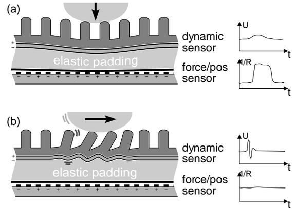
Fig. 4: **Principle of simultaneous force/position and slippage detection:** The combination of a PVF<sub>2</sub> sensor (upper layer) with a “tonic” piezoresistive sensor material (lower layer) allows reliable discrimination between static pressure (a) and slippage (b).
